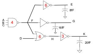
Problem 3 A segment of a logic block is shown below. Assume the lengths of all devices are L<sub>MIN</sub>. Assume all gates are sized for equal worst-case rise and fall times.
