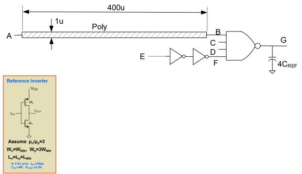
Problem 7 Assume a process has Poly with two different sheet resistances as shown below. Assume the capacitance density to substrate of both Poly layers is  $800aF/\mu m^2$ . Determine the propagation delay from A to G. Assume the gates in the process are characterized by a minimum length reference inverter with
